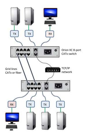
Structure of a matrix grid network
