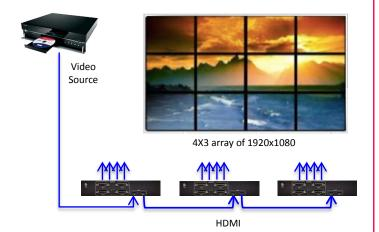
Using cascading feature to implement 4x3 video wall
