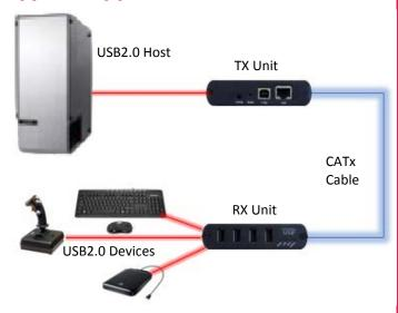
The CrystalLink USB2.0 CATx is ideal for use in commercial, industrial, residential, medical, data center, and other environments where multiple USB devices need to be connected at distances up to 330 feet (100m) away from a host PC.
